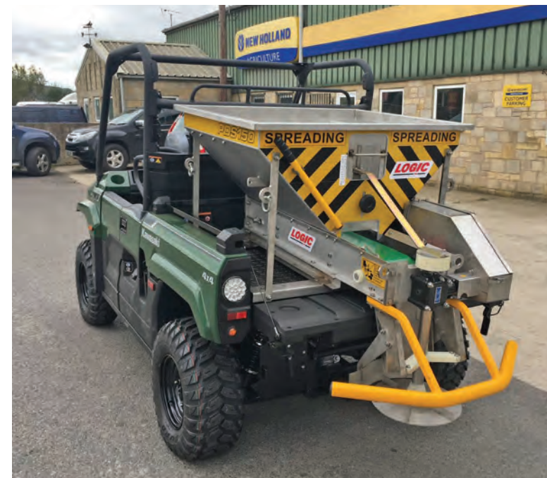
Top: The Logic GDS150 salt spreader – designed for towing. Above: This Logic PDS150 variant is designed for mounting on the rear platform of UTVs, pick-ups, 4x4s or three-point linkage compact tractors.
