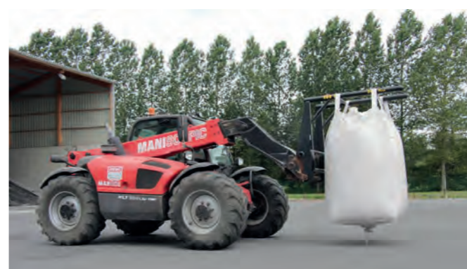
The Big Bag Handler is a strong tubular structure with a lifting capacity up to 2,400kg (four loading points each with 600kg capacity).
