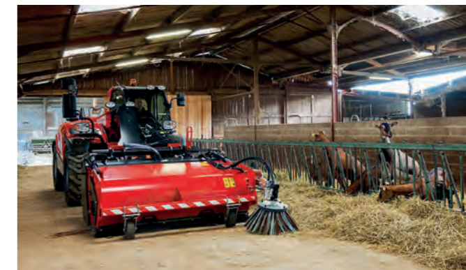
The Pickup Sweeper will clean up to 2500m 2 in 10 minutes, sweeping and collecting in one operation even where the ground is not flat.
