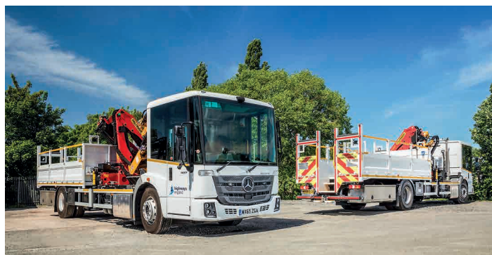
Built on a Mercedes-Benz Eonic 18-tonne chassis, the barrier rigs have been fitted with Palfinger PK190001.SLD5 cranes and Orteco HD 800 pile drivers.
