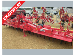
REF: H1110778 Pöttinger Lion 6000 Power Harrow, 6m folding width for tractors up to 270hp £25,000
