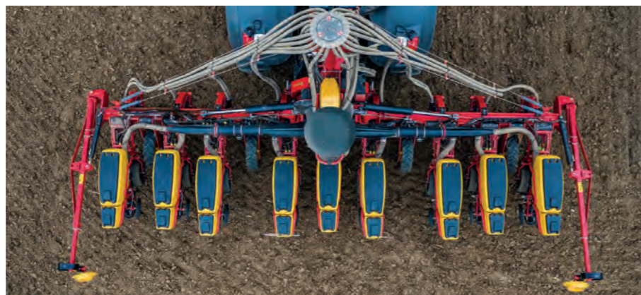
The Väderstad Tempo WideLining system is designed for working in a standing silage maize crop and will automatically adjust the row units to create tramlines based on the working width of the liquid manure spreader
