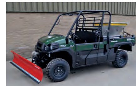
A PDS150 salt gritter mounted into a Kawasaki Mule, also fitted with an electrically operated Logic snowplough.
