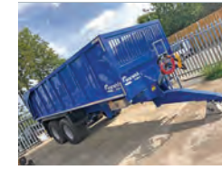
Warwick WB14FM 14-ton grain trailer, 4mm floor, 3mm sides, air/hyd brakes, ABS, hydraulic tailgate, £18,415
