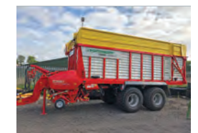
Pöttinger Torro 6010L combiline loader wagon, steering axle, knife bank with 45 durastar knives £69,250
