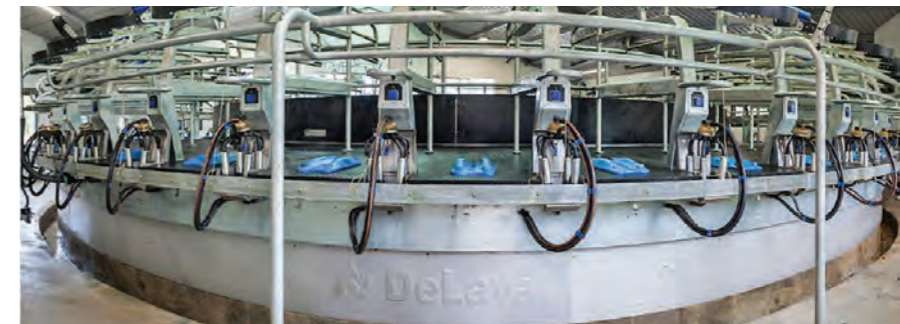
DeLaval's new E100 rotary milking parlour improves conditions and reduces labour requirements.
