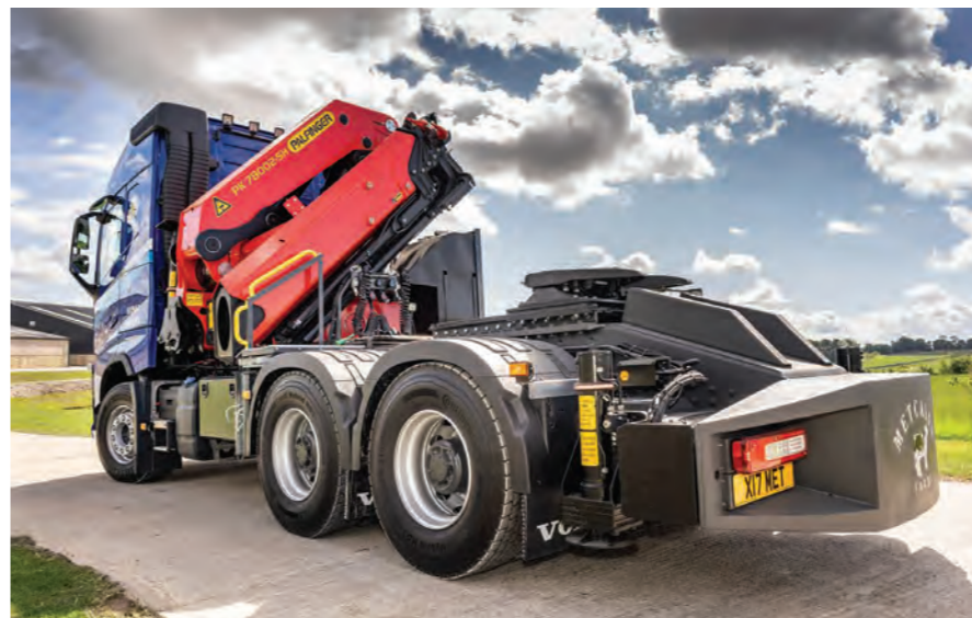
The extensively modified Volvo FH 64T tractor fitted with a Palfinger PK78002-SH crane.
