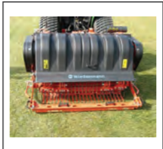
Wiedenmann SL6 Terra Spike £14,250. Deep aeration and removal of compactions up to 21cm depth, exchangeable tine holders, rear roller, VibraStop.
