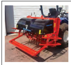
2014 Wiedenmann G160 Terra Spike, £11,500. EX-HIRE, deep aeration and removal of compactions up to 270mm, 1.6m width, manual depth control.
