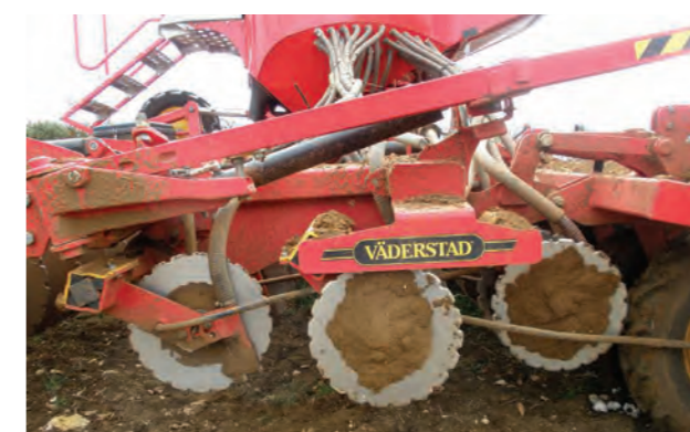
Three rather than two banks of coulters discs enables the 8m Vaderstad Rapid to cope with more trash in wetter soils
