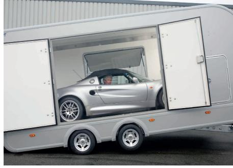
ground clearance an optional pair of ramp skid extenders are available
