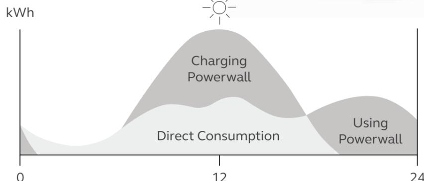
Tesla Powerwall is charged at times of high solar exposure, enabling you to spread the availability of your solar energy across a 24 hour period.
